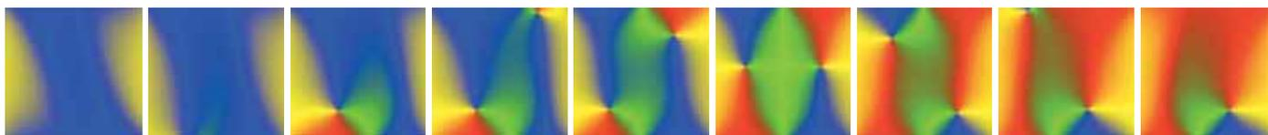
**Figure 4: The critical points along a minimum energy path (path b) followed by the magnetization during the switching of the element. The color code indicates the direction of the magnetization.**
